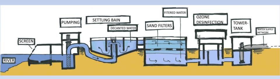
SETTLING BASING (SETTLING POND-DECANT POND)
